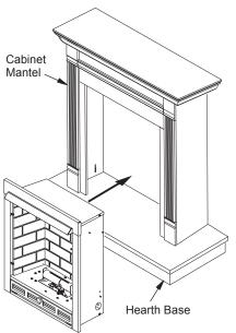
Figure 12 - Installing Fireplace into Mantel Assembly
